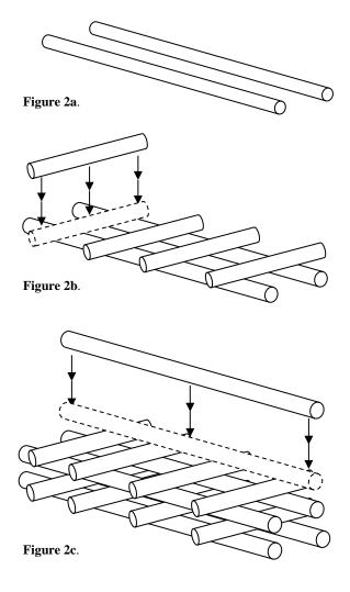
**Figure 2.** Stages of deadwood fence construction; a) two long 'rails' are laid parallel about 1m apart, b) shorter 'sleepers' are laid perpendicular on top of the rails, spanning the gap and creating a second layer, c) the fence is built up in alternating layers of rails and sleepers
